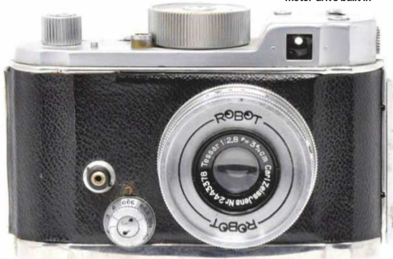
Robot II, with clockwork motor drive built in
